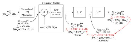
We also can bring the frequency shifter before all the non-linear devices and therefore reduce the frequency of the required oscillator to the minimum value by finding the required carrier frequency at the input of each non-linear device to insure that the carrier frequency of the final output of non-linear devices is the desired final carrier frequency.
